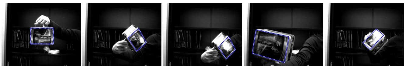
Figure 8. Video 5: A metallic box is tracked under large changes in rotation and scale while experiencing high specular reflections.
