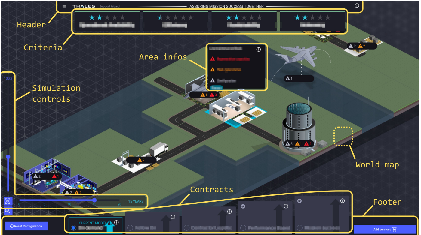
Figure 10: Support Wizard application main window. Each annotated section of the GUI represents a Bloc class augmented as a component.
