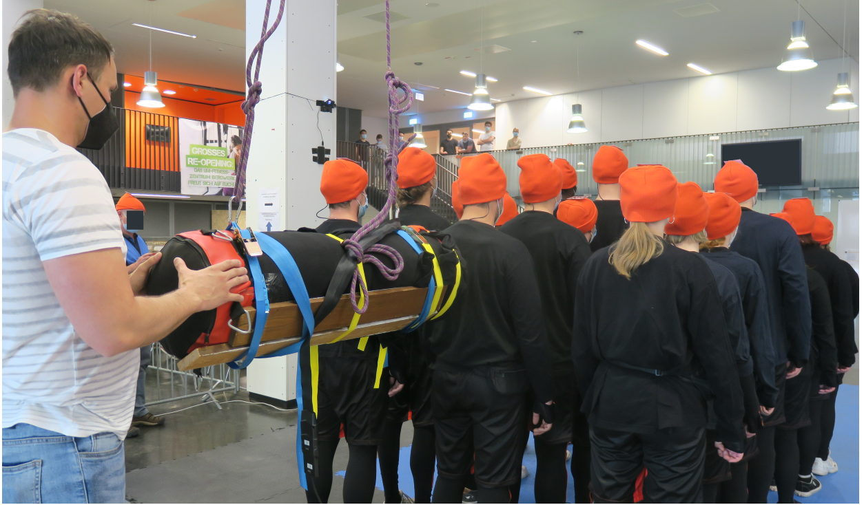
Figure 2: Picture of the experiment for a group formation close to the 4B55 configuration. In this picture, the group is only composed of participants wearing motion capture suites. For the 4B55 configuration, additional participants without motion capture suites were placed on the side boundaries of the group formation.
