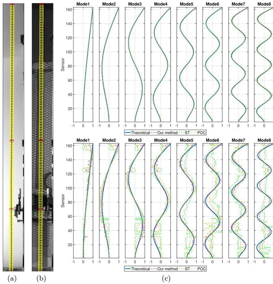
**Fig. 2.** Video frame including 163 regions of interest (ROI) with (a) clean and (b) unclean background. The red boxes are ROIs corresponding to laser sensing positions, while others without laser are marked yellow. (c) First 8 mode shapes of beam obtained by finite element analysis and vision algorithms in conditions without (upper) and with (lower) illumination variation and unclean background.
