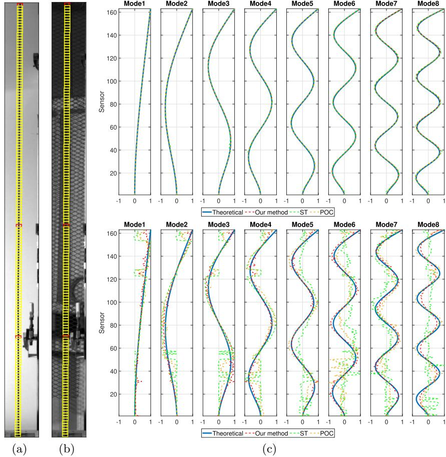
**Fig. 2.** Video frame including 163 regions of interest (ROI) with (a) clean and (b) unclean background. The red boxes are ROIs corresponding to laser sensing positions, while others without laser are marked yellow. (c) First 8 mode shapes of beam obtained by finite element analysis and vision algorithms in conditions without (upper) and with (lower) illumination variation and unclean background.
