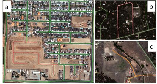
**Fig. 3.** Road materials classification examples. Green for processed roads and red for unprocessed roads (a), pink for gravel roads (b) and orange for sand roads (c).
