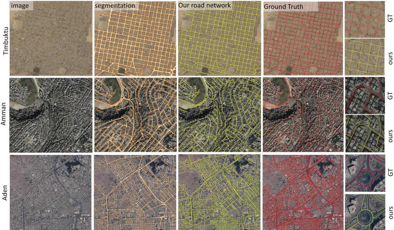
**Fig. 4.** Road networks generated by our pipeline over Timbuktu, Amman and Aden (top to bottom rows), with input satellite images, road segmentation, our extracted road networks, the Ground Truth, and crops (left to right columns). In the crops, Ground Truth are marked in red and our results in yellow.
