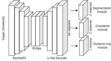
**Fig. 2.** The proposed new architecture for road segmentation from a single satellite image.
