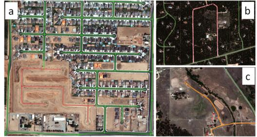
**Fig. 3.** Road materials classification examples. Green for processed roads and red for unprocessed roads (a), pink for gravel roads (b) and orange for sand roads (c).
