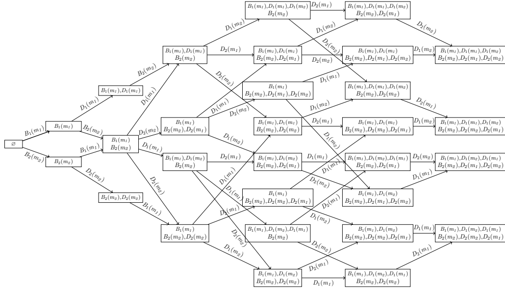
■ Figure 11 Set of states S as a state graph obtained from the histories of the system in Algorithm 4. Events are abbreviated for clarity: B_i(m_i) and D_i(m_j) are short for B.r\_broadcast_i(m_i, i).inv and B.r\_deliver_i/(M_j, j, j).res , respectively. The states in which a process receives a message before invoking r\_broadcast , the B.r\_broadcast_i(m_i, i).res events, and the event indices are omitted for clarity.
