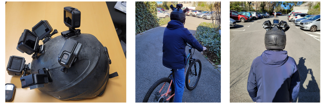
Fig. 9. Left: Our 6-GoPro HERO6 camera helmet rig. Middle: We performed captures on a bicycle at 6–7 km/h and (Right) on foot.
