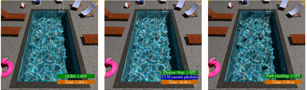
Fig. 9. Comparison between our algorithm (left) and Photon Mapping (center) and Practical Path Guiding without denoising (right). Both methods render good quality caustics; our algorithm is much faster for the caustics on this specific scene.
