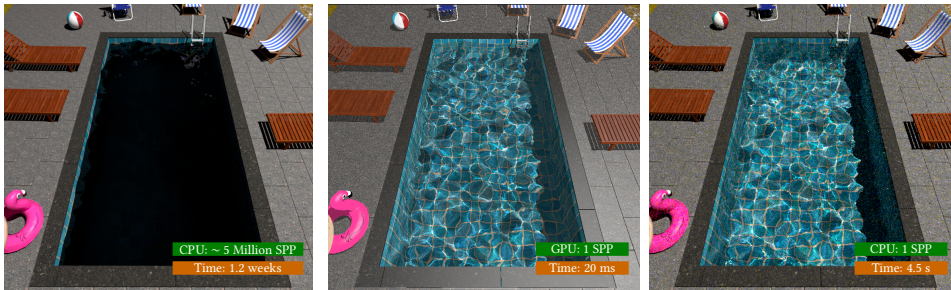
Fig. 1. Refractive specular surfaces, like the water surface in this pool, create caustics. Classical path-tracing (left) cannot find a path connecting the bottom of the pool and the point light source, and fails at rendering these caustics. Manifold exploration methods (right) work but are not compatible with interactive rendering. Our method (center) runs interactively, by reducing the space where it searches for solutions to a curve.
