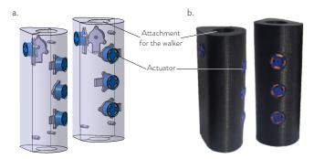
**Fig. 1.** Right and left haptic handles designed for providing directional tactile sensations. a) Computer-Aided Design (CAD) of the 3D-printed handle, made from flexible TPU material, featuring alcoves to house the actuators in a "T" - shape configuration. This design naturally stimulates the thumb, the second metacarpal bone of the palm, and the index finger. b) Image of the two symmetrically designed handles [17].
