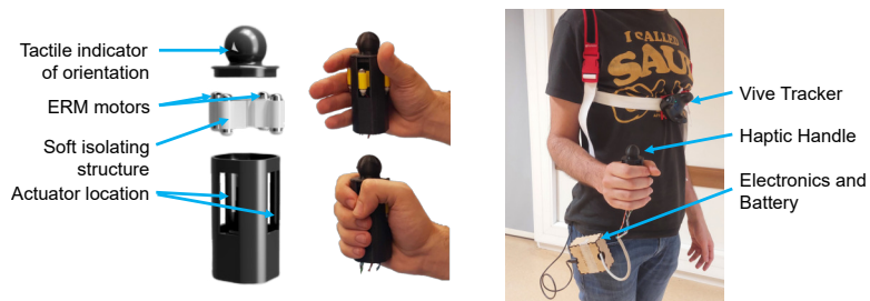
Fig. 1. Our custom haptic handle provides localized vibrotactile feedback within the user’s hand thanks to four ERM actuators isolated with a soft 3D-printed structure (left). We evaluated three navigation strategies with two haptic rendering schemes, having participants follow three invisible target paths using the haptic navigation information provided by the haptic handle (right).
