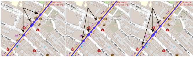
Fig. 2: Hypothetical trips—moving from top to bottom—along a path getting stopped at an intersection. The three arrows point towards three distinctive groups (the two extrema and the middle pack). Left: The three groups are evenly spaced on the path. Middle: The first dot has to stop at the intersection and the middle pack thus catches up. Right: The middle pack is now stopped, the first dot moves on, and the last dot catches up.
