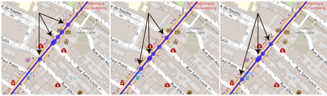
Fig. 2: Hypothetical trips—moving from top to bottom—along a path getting stopped at an intersection. The three arrows point towards three distinctive groups (the two extrema and the middle pack). Left: The three groups are evenly spaced on the path. Middle: The first dot has to stop at the intersection and the middle pack thus catches up. Right: The middle pack is now stopped, the first dot moves on, and the last dot catches up.
