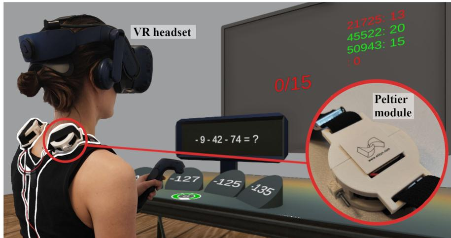
**Fig. 1.** Participants were immersed in a virtual room where they answered arithmetic questions for 5 minutes. During this period, the two Peltier modules strapped to their backs either warmed up, cooled down, or stayed neutral.
