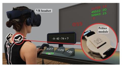
Fig. 1. Participants were immersed in a virtual room where they answered arithmetic questions for 5 minutes. During this period, the two Peltier modules strapped to their backs either warmed up, cooled down, or stayed neutral.
