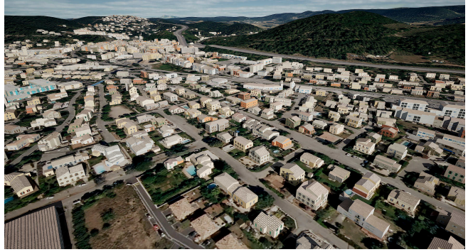
Figure 7. Textured reconstructions of Le Luc, France. Both airborne Lidar point clouds and cadastral maps available online [13] were used as input to generate 3D building models, prior to the texturing process. Best viewed in electronic version.
