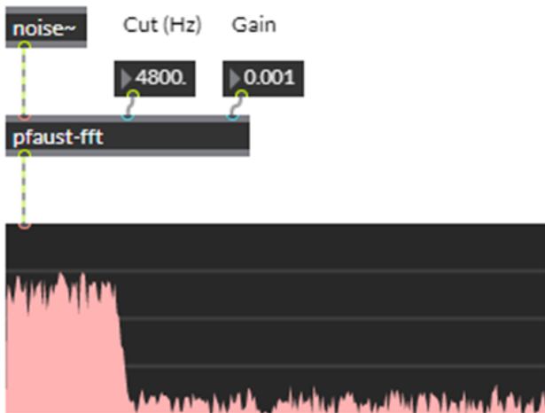
Figure 6: Spectral high-shelf filter running in JSPatcher.
