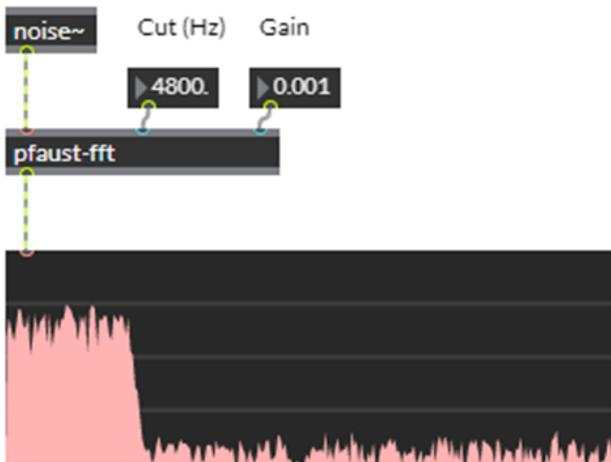
Figure 6: Spectral high-shelf filter running in JSPatcher.
