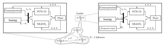
Fig. 1. Control schemes for the multi-robot team. Starting from the building blocks necessary to run the connectivity-maintenance control (communication, inter-agent and environmental sensing), we control the team motion either through the standard model-based GCM approach or the proposed ML-based NRANN one. The objective is to evaluate the pros and cons of employing GCM vs. NRANN for the control of multi-robot systems.
