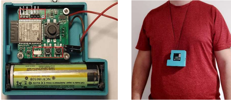
Fig. 3. 3D Printed Enclosure, 18650 Li-ion battery and hardware of the fall detection device. The areas with the red frame are used for easier programming of the device but they can be skipped, if we would like to minimize the PCB size.
