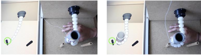
Figure 15: The goal position is illustrated by a green circle in both figures. On the left, the obstacle is not modeled in the inverse model. The obstacle prevents the real robot from reaching the goal. On the right, however, contact with the obstacle is taken into account in the inverse model, enabling the real robot to find a solution to the inverse problem of reaching the goal position while sliding over the obstacle. Figures from [5]
