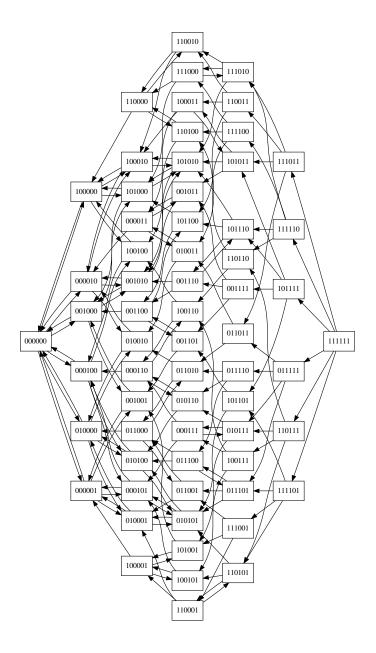
Figure 5: Communication graph for ECA 9-AEGH. An arrow between two configurations indicates a potential transition of the system. Self-loops are removed for the sake of clarity. Note that recurrent states are the configurations which do not contain two consecutive 1's.
