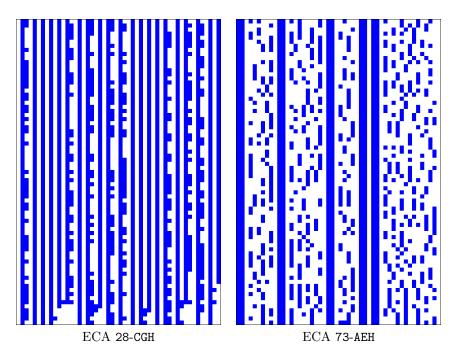
Figure 6: Space-time diagrams of ECA 28-CGH (type B2) and ECA 73-AEH (type B3).
