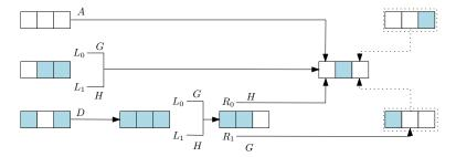
Figure 2: Transition from different blocks of states xyz to block 010 with active transition A, D, G, and H. White and blue box represent cells in states 0 and 1 respectively.
