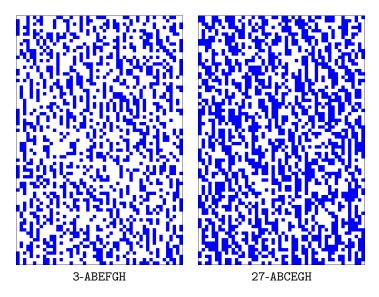
Figure 1: Space-time diagrams of ECA 3-ABEFGH and 27-ABCEGH (type A1) for a size n=50. White and blue squares represent cells in states 0 and 1, respectively. Time goes from bottom to top and each line represents the state of the automaton after n random updates. This convention is kept in the rest of the text.
