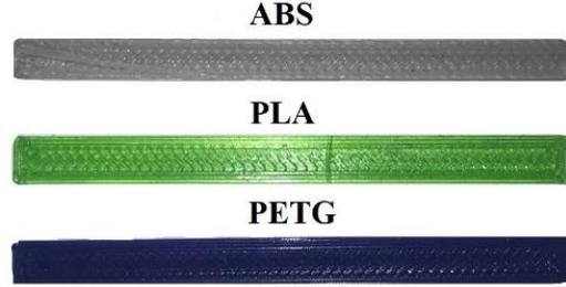
**Fig. 7.** Specimens made of FDM technology and ABS, PLA and PETG materials
