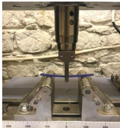
Fig. 6. Three-point bend with Tensile machine SHIMADZU
