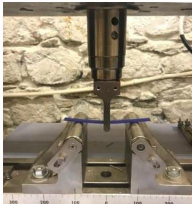
**Fig. 6.** Three-point bend with Tensile machine SHIMADZU
