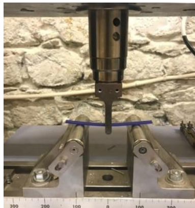
Fig. 6. Three-point bend with Tensile machine SHIMADZU
