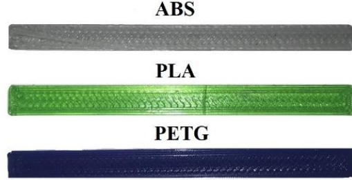
Fig. 7. Specimens made of FDM technology and ABS, PLA and PETG materials The calculation of the Young's modulus was done using the equation
