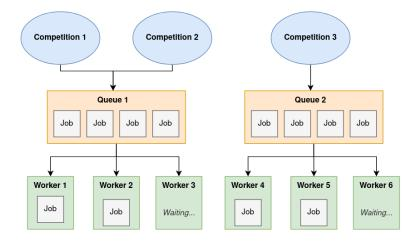
Figure 3: Diagram of the structure of workers and queues. The queues dispatch the jobs between the compute workers. Note that a queue can receive jobs (submissions) from several competitions, and can send them to several compute workers.
