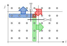
Figure 3. Flow-out set of a tile intersected with each consumers tile's flow-in set. The breakup we propose splits iterations that have different consumer tiles.
