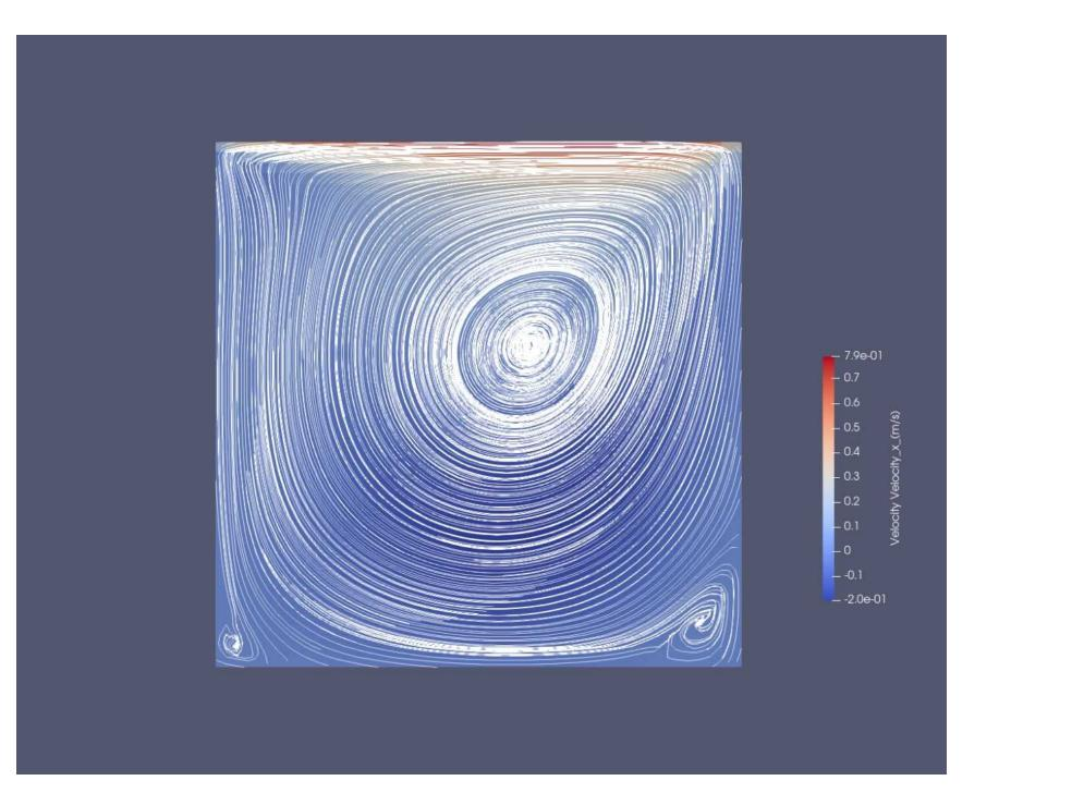
We converged to a stationary state with **viscosity** that was also implemented in the manner of the previous paragraph, we can observe the formation of vortices, which is not guaranteed by classical schemes at Low Mach numbers
