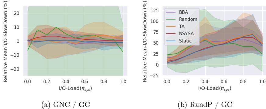
Fig. 3: Relative Mean-I/O-SlowDown for different algorithm combinations when I/O-load( $\pi_{\text{sys}}$ ) increases. Placement are compared with GC. Lines show the mean value, and the area around them is the percentile interval ( $10^{\text{th}}$ - $90^{\text{th}}$ ).
