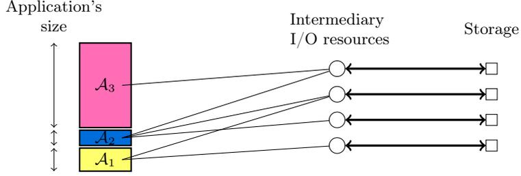
Fig. 1: Representation of the architecture: three applications  $\mathcal{A}_1$  (resp.  $\mathcal{A}_2$ ,  $\mathcal{A}_3$ ) use two (resp. three, one) I/O resources. The number of I/O resources is not necessarily correlated to the size (number of compute nodes) of the application.
