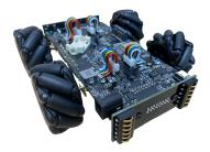
Figure 1: Current Version of the FreeBot with Mecanum Wheels and Front/Rear charging ports (152x133x48mm)
