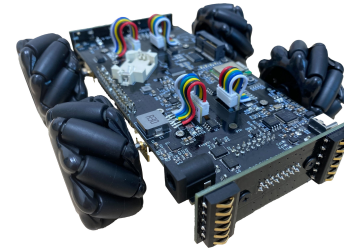
Figure 1: Current Version of the FreeBot with Mecanum Wheels and Front/Rear charging ports (152x133x48mm)
