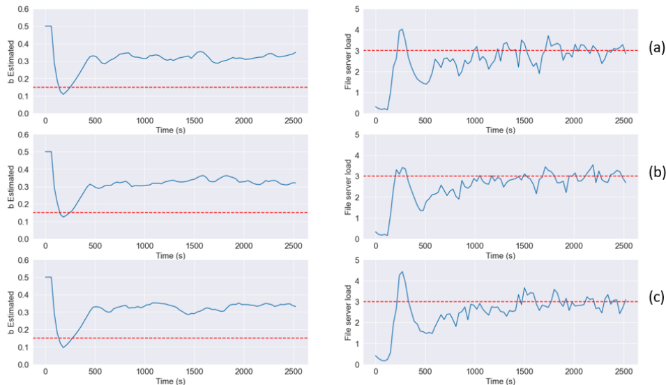
Figure 4.12: Outcomes based on variations in initial Covariance values. Figure (a) corresponds to an initial condition of 100, while Figure (b) employs an initial value of 10^4 , and Figure (c) utilizes 10^6 as its starting point.
