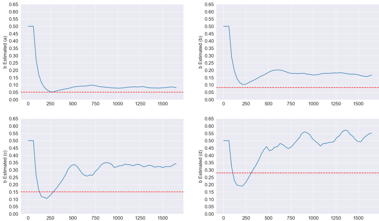
Figure 4.18: Zoomed-in estimation results prior to the disturbance's arrival. In picture (a), we observe the scenario with a data size of f=50 MByte. In picture (b), the scenario with f=100 MByte is depicted, in (c), the scenario with f=200 MByte is presented, and in (d) the case with f=400 MByte .
