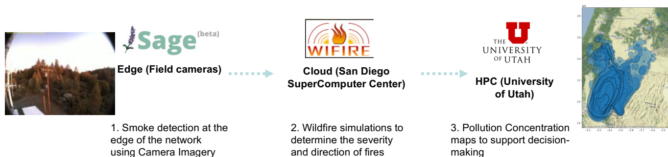
Fig. 1: Monitoring and managing the air quality impact of wildfires – This driving urgent application usecase is designed using R-Pulsar to composed sensors provided by the SAGE platform align, wildfire data and model provided by the WIFIRE platform along with local pollution concentration maps, all distributed across the computing continuum.
