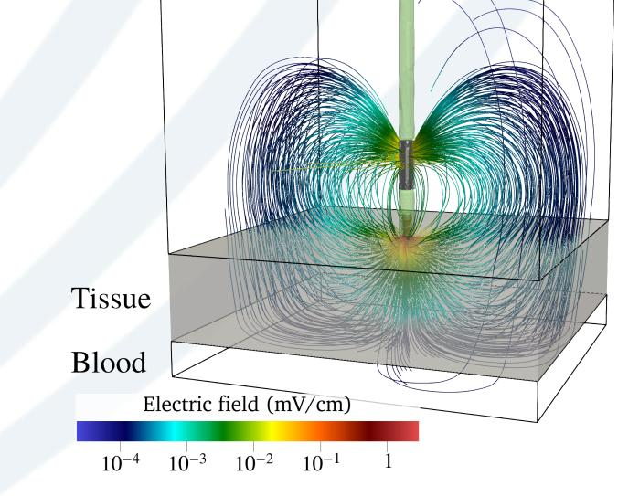
• Fig. 7. 3D computation of the electric field generated by the pacemaker in the tissue and blood. The lead geometry, including screw and ring, is as realistic as possible and based on manufacturer's CAD.
