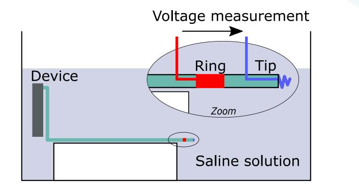
**Fig. 5.** Sketch of the bench test used to calibrate the electrode contact models.
