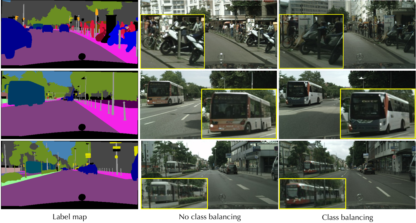
Figure S5. Qualitative examples of images generated with and without balanced sampling to train models on Cityscapes.
