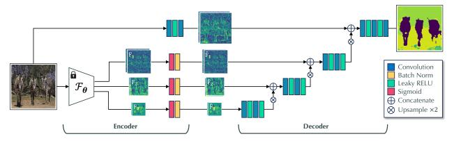
Figure 2 Architecture of our discriminator model. The encoder consists of a pre-trained feature backbone  $\mathcal{F}_{\theta}$  (left), residual blocks at full image resolution (top), and trained feature decoder that aggregates the multi-scale features from the frozen backbone (right).
