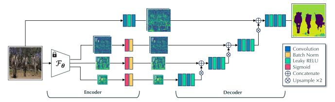
Figure 2. Architecture of our discriminator model. The encoder consists of a pre-trained feature backbone  $\mathcal{F}_{\theta}$  (left), residual blocks at full-image resolution (top), and trained feature decoder that aggregates the multi-scale features from the frozen backbone (right).
