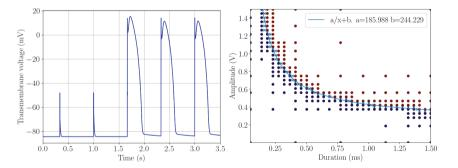
**Fig. 5.** Transmembrane voltage (left) computed for a single set of parameters  $(V_{\text{stim}}, d, S, g_{\text{e}})$ ; and Lapicque curve (right) obtained after detection of a 50% capture ratio. Blue points are for 0% capture, and red points for 100% capture. (Color figure online)
