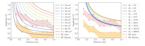
**Fig. 6.** Comparison of Lapicque curves (solid lines) computed with different values of S (left) and  $R_1$  (right). The shaded regions indicate where the experimental capture threshold is located, for different stimulation sites on the tissue wedge.
