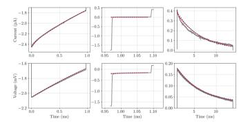
**Fig. 4.** Fitted currents and voltages when calibrating parameters  $\theta = (R_1, R_2, \tau_1, \tau_2)$ . Gray solid lines are one experimental dataset, blue dotted lines are computed with  $\theta$  calibrated with this dataset, and red solid lines from the calibration of the 9 datasets together. (Color figure online)
