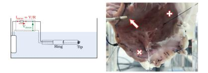
**Fig. 3.** Left: sketch of the bench test used to calibrate the electrode contact model. Right: right ventricle endocardial view of the tissue wedge preparation with the pacemaker electrode implanted in the septum (pointed by arrow). Other implantations sites were located in the apex  $(\times)$  and at the base of the ventricle (+).
