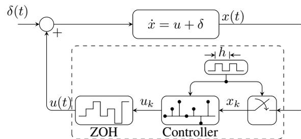
Figure S5: Closed-loop system. The state of the continuous-time dynamics is sampled every  $h$  seconds. Such information is used for computing the control input  $u_k$  which passes through a classical zero-order-hold mechanism to obtain the feedback input signal  $u(t) = u_k$  for  $kh < t \leq (k + 1)h$ .
