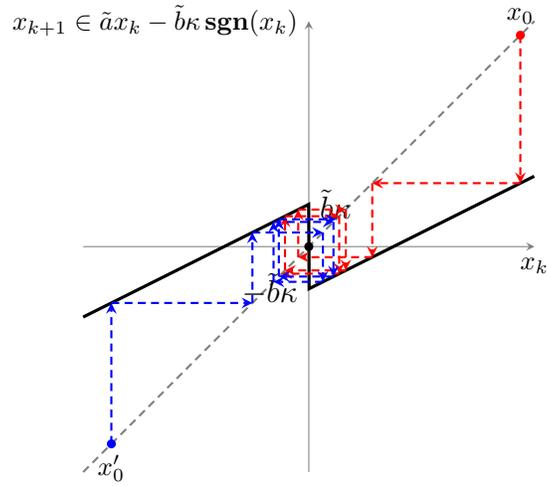
Figure S2: Cobweb diagram of (6) with parameters:  $\tilde{a} = 0.5$ ,  $\tilde{b}\kappa = 0.75$  for two different initial conditions. The explicit discretization of the set-valued law (2) yields an iteration with a non-monotone map, such that for almost all initial conditions, the closed-loop shows an oscillatory behavior. The amplitude of the oscillation is proportional to the control gain  $\kappa$ .
