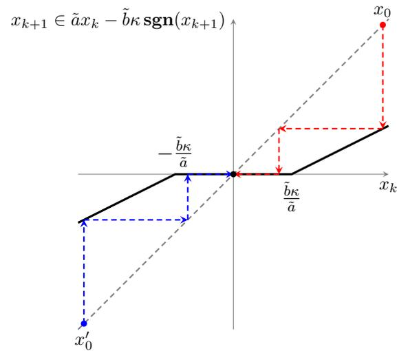
Figure S3: Cobweb diagram of (8) with parameters:  $\tilde{a} = 0.5$ ,  $\tilde{b}\kappa = 0.75$ . The implicit discretization of the set-valued law (2) yields an iteration with a maximal monotone map, such that for any initial condition the state converges towards the origin after a finite number of steps.
