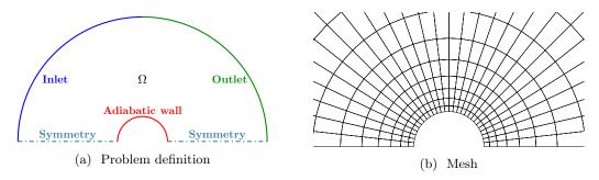
Figure 10: Geometry, boundary conditions and mesh for the case of the axisymmetric flow past a sphere.
