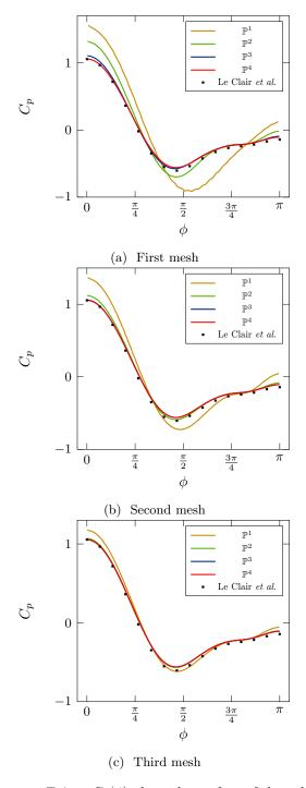
Figure 16: Pressure coefficient  $C_p(\phi)$  along the surface of the sphere at  $\mathrm{Re}_d=200.$
