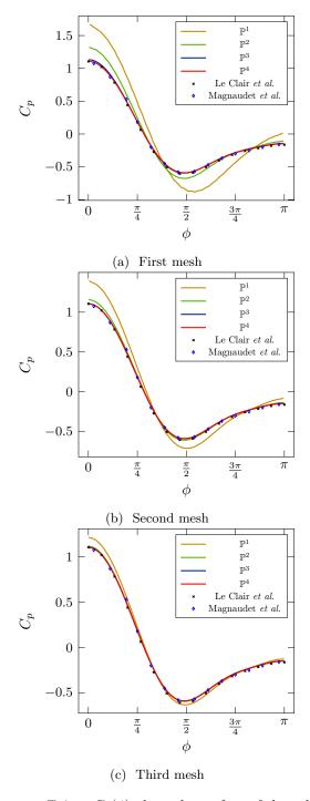
Figure 13: Pressure coefficient  $C_p(\phi)$  along the surface of the sphere at  $\mathrm{Re}_d=100.$
