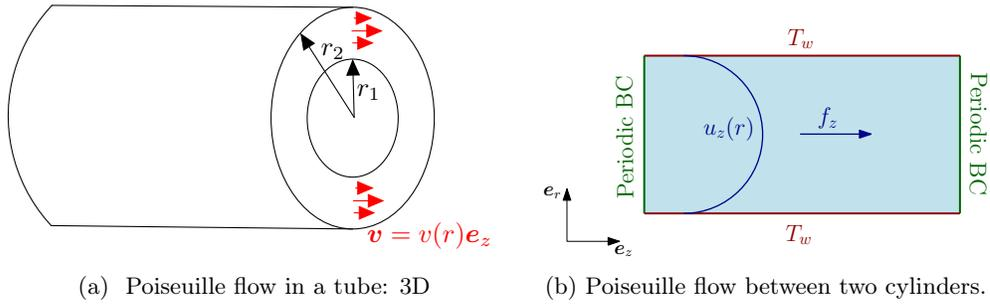
Figure 5: Poiseuille flow between two cylinders - Problem definition.
