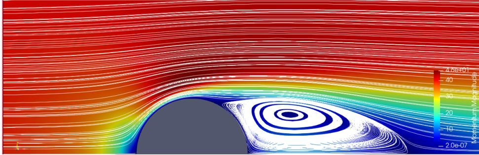
(a) Momentum magnitude and streamlines near the surface of the sphere, with a visible recirculation zone.
