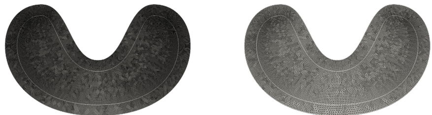
Figure 7. Representation of the mesh of \Omega with 56193 degrees of freedom (left) and with 14169 degrees of freedom
