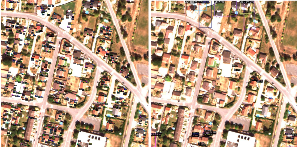
Figure 19: Example of roof section corners inference directly on a raster image of size 768 \times 768 , with ground truth on the left, and result output on the right. The large number of roof sections in the ground truth overloads the Mask-RCNN algorithm.
