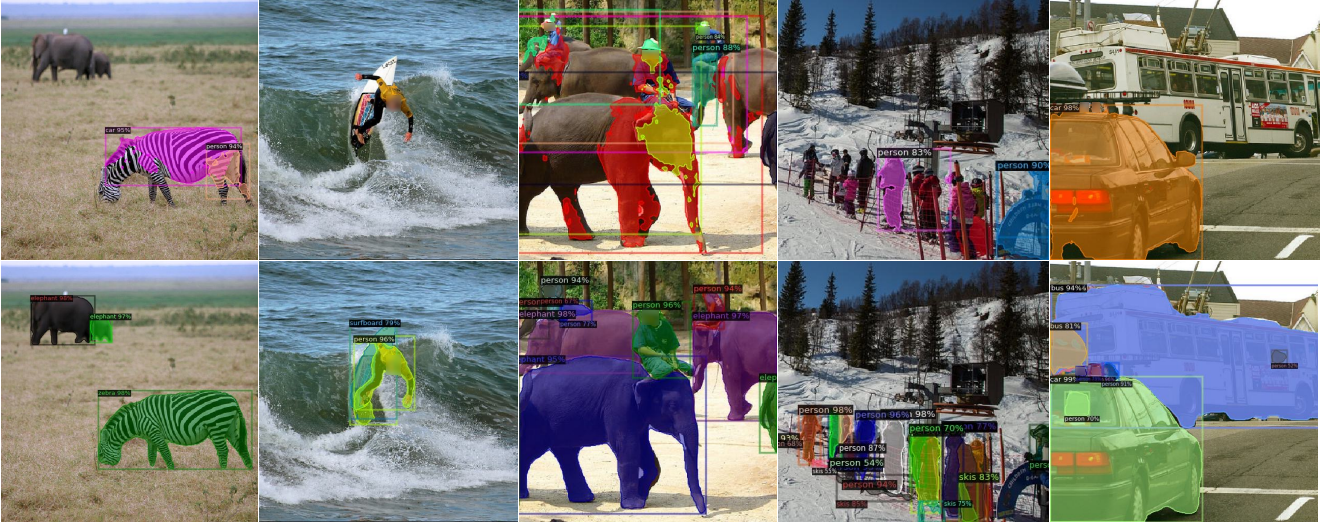
Figure 2. Results on the COCO dataset when using from 5% labeled data, with supervised training (top) and our semi-supervised approach (bottom). Our approach leads to more detected objects that are segmented with higher accuracy. Results best viewed by zooming in.
