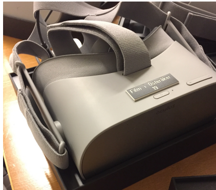
Fig. 1. The HMD Oculus Go. Multiple devices were used, and they were connected through the Showtime VR application, controlled by nurses using a tablet or smartphone.
