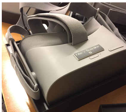
Fig. 1. The HMD Oculus Go. Multiple devices were used, and they were connected through the Showtime VR application, controlled by nurses using a tablet or smartphone.
