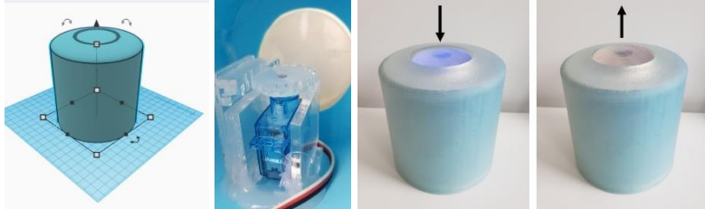
Fig. 6. Luna: 3D-printed shape-changing desk object as P6’s design with an emerging light that moves up slowly and changes its ambient light as break time approaches.
