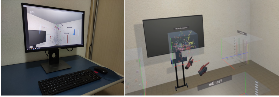
Fig. 5. The virtual room had a TV that showed the tasks. The participants started the exploration in the middle of the room, and the visualizations were displayed around them. Users interacted with the visualizations using keyboard + mouse (left), while in the VR environment they used controllers as virtual hands (right).
