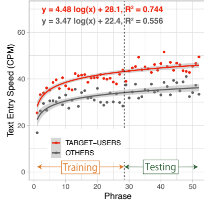
Fig. 11. Average JoyFlick text entry speeds of TARGET-USERS and OTHERS. The gray bands show 95% confidence interval.
