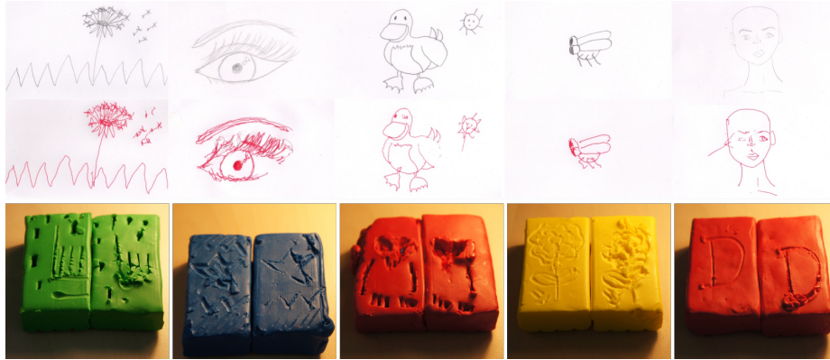
Fig. 9. Examples from the user study. The top row shows five drawing examples (top: participant, bottom: robot arm). The bottom row shows five modelling examples (left: participant, right: robot arm). Some artifacts, like the missing part of the duck, originated from calibration problems, others, like the additional lines in the most left and most right image, from the trajectory editing during the study.
