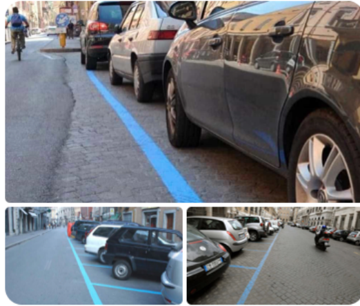
Fig. 1. Parking place types: parallel (top), angle (bottom left), perpendicular (bottom right)
