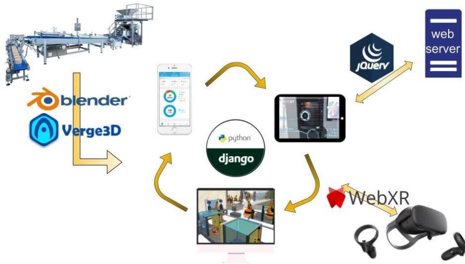
Fig. 1. The developed framework and workflow for the building of a digital twin.
